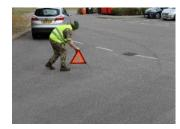
If you find yourself on a road then you need to make sure that the vehicle is out of the way of other traffic and that a warning triangle is placed at least 45m behind the vehicle. To make yourself more visible, wear a Hi-Vis jacket if possible.
